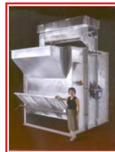
Bucket elevator boot 1200MT
