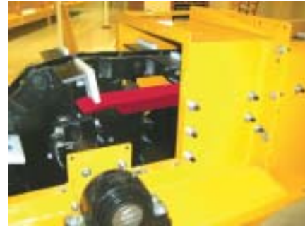
Fig.2: A chain lift-off utilizing the flight to remove the chain from the sprocket.
